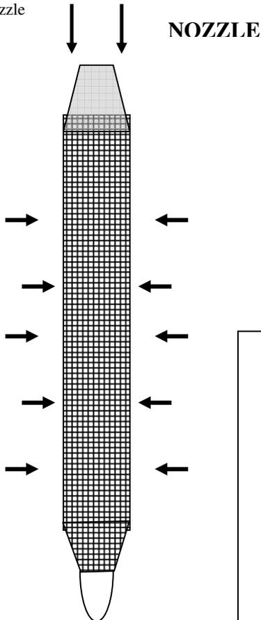
3. Squeeze Sampler & release multiple times to release air and expand volume. Add water & repeat as needed to fill.
